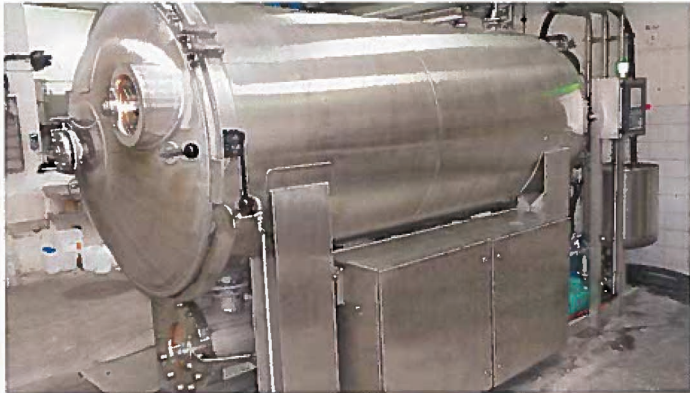
Lab-Pro's Dyewa machine features a rotating perforated beam whereby the dye bath is sprayed from the interior of the beam onto the fabric wound on the beam.
